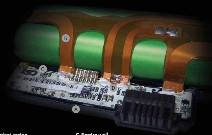
A. Fire-retardant casing B. Flexible circuit interconnects
